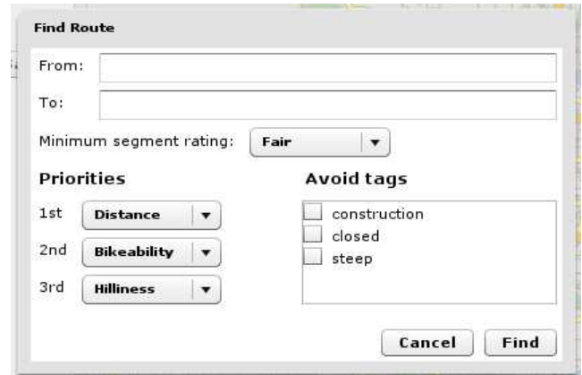
Figure 2. Our current automatic route finding interface. Edge weight is calculated as a weighted sum of the (normalized) priority factors.
